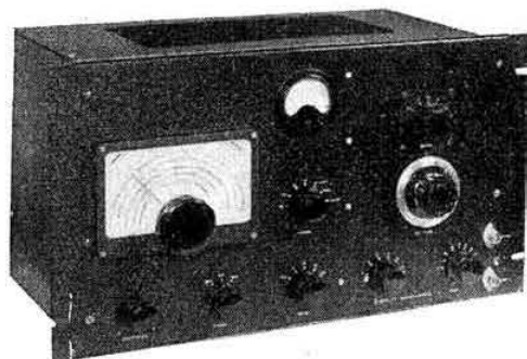
Front view of the Elizabethan all-band 150 W transmitter showing the neat arrangement of the controls. From left to right (bottom row), excitation (drive), variable power control, exciter band-switch, coarse loading and fine loading (as used in model shown). Above (left to right), v.f.o. tuning, meter switch and p.a. tuning, with the p.a. band-switch above.
